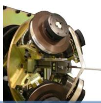
**Automatic Turn Taping Machine (ATTM)**
